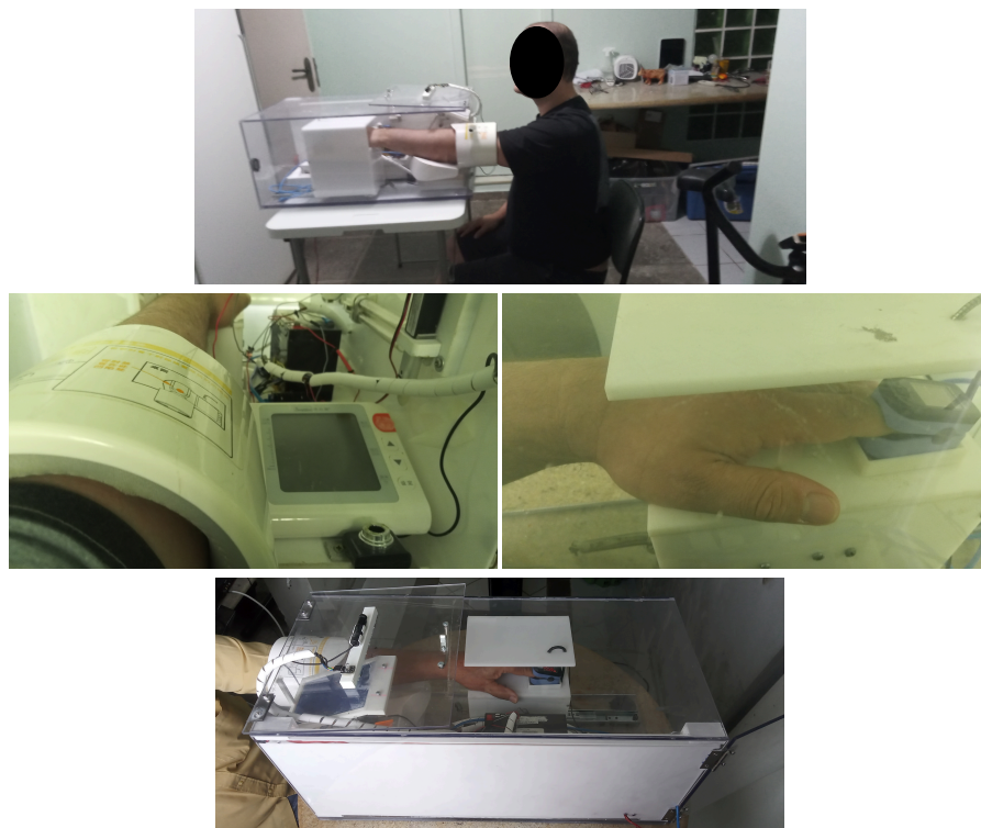
Figure 12 – Illustration of arm and hand placement for data collection using the IPMA equipment.
