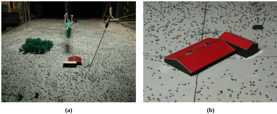
Figure 5-2: (a) Wind tunnel test section with the building model and (b) close view of the pig barn model used in the wind tunnel.
