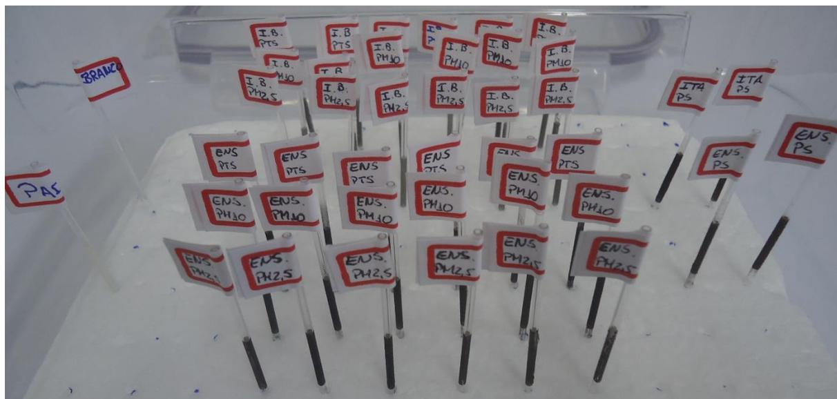
Figure 18. PM samples into capillary tubes for RSr-XRD analysis.
