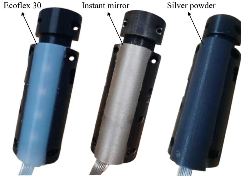
Figure 9 – Ecoflex 30 OS version with the new reflective coating layers.
