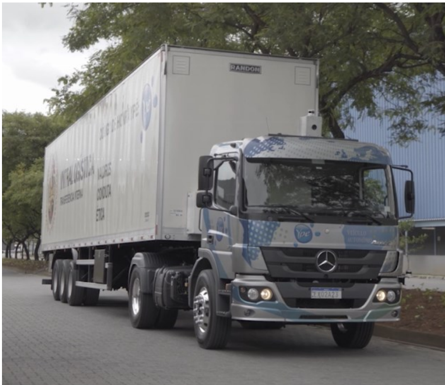
Fig. 28. Mercedes-Benz truck used for logging odometry and sensor readings at the industrial plant.
