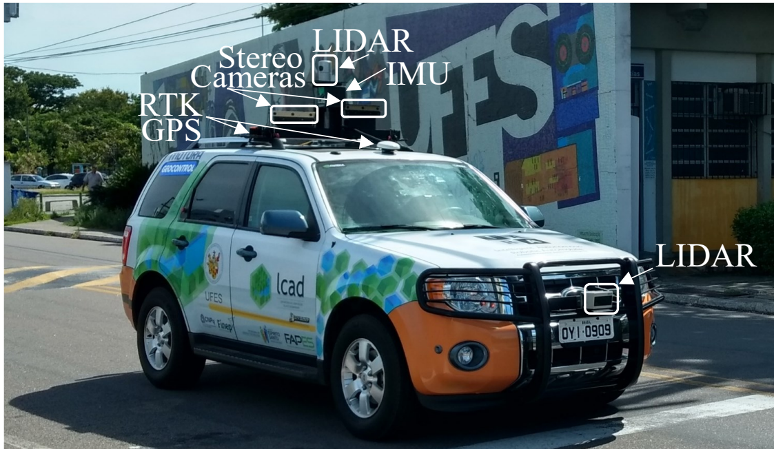
Fig. 3. The Intelligent Autonomous Robotic Automobile (IARA) of LCAD/UFES. IARA uses several sensors to build an internal representation of the external world. A video of IARA's autonomous operation is available 4 .
